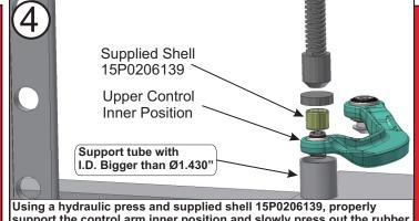
support the control arm inner position and slowly press out the rubber bushing with bonded outer metal casing with supplied shell. Be sure the shell is centered evenly into the control arm.
